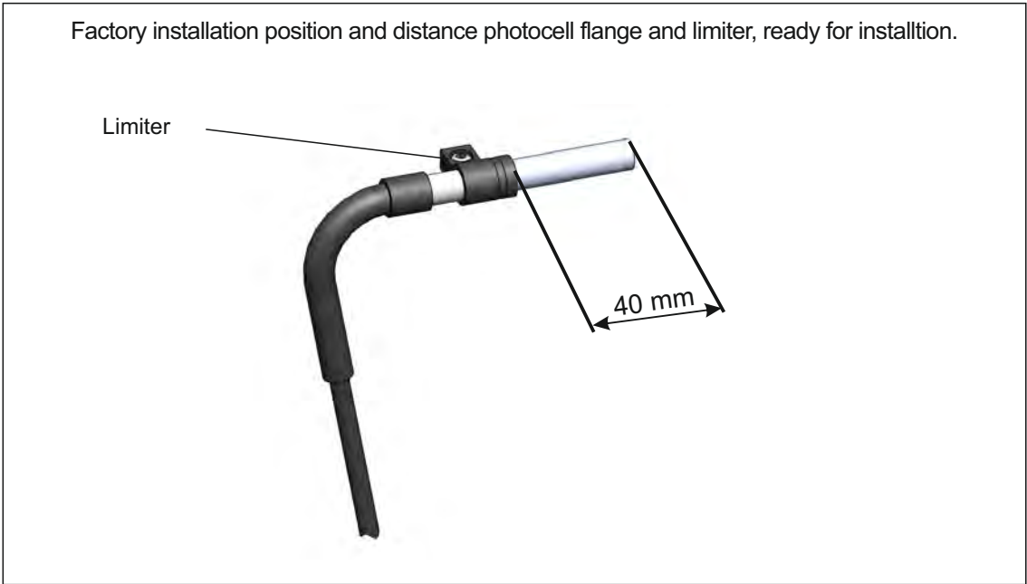
Carefully install photocell into flange on the box to the limiter (so it clicks)
